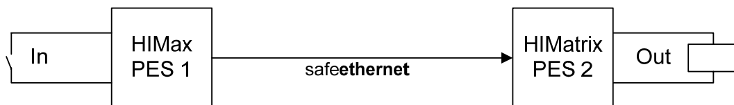
Figure 5: safeethernet Connection between One HiMax and One HiMatrix Controller
