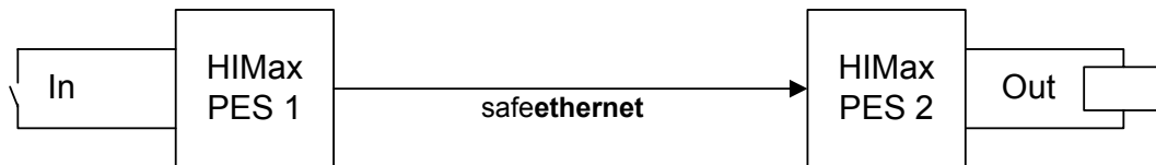
Figure 4: safeethernet Connection of Two HiMax Controllers
