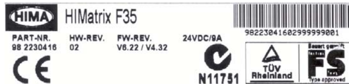
Figure 10: Type label of a HIMatrix F35 controller
